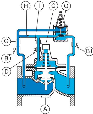
As long as upstream pressure is below the setting pressure, pilot (Q) is closed, upstream pressure pushes on the membrane of the main valve (A) which keeps closed.
