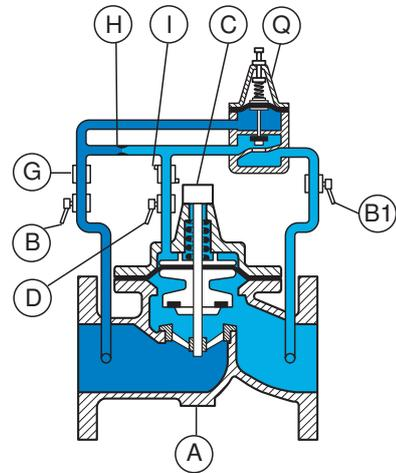
As soon as upstream pressure is getting higher than setting pressure, pilot (Q) opens, releases the pressure from the membrane of the main valve (A) which opens and releases the overpressure.
